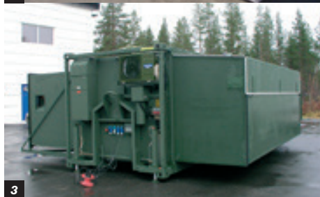
2. Expandable ISO 10' shelter for Link 16, expanded.
